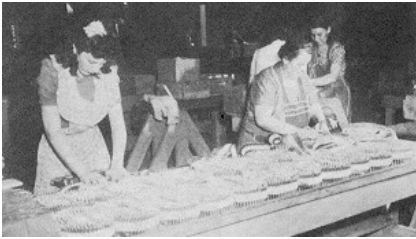
.50-caliber machine gun ammunition in fabric belts are being prepared for crating in 1941. Fabric belts would gradually give way in 1945 to steel links.
